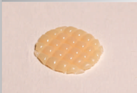
Microrelief of ReLight composite uncured surface after 20 min at 37°C
